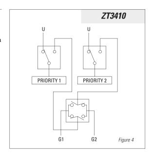
selector switch. When a utility failure occurs, both gensets are started and the first available unit feeds the critical load through automatic operation of the power selection switch. The second generator, if required, operates to feed the secondary load. If the alternate genset is not required, it will run on a 5 minute verification timer and shut down. (Figure 4)
